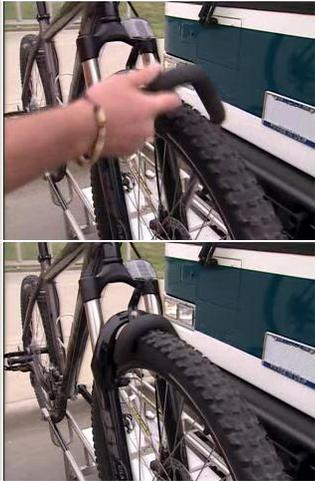
5. When your bike is loaded, lift the support arm and raise it up over the front tire so the hook rests on the highest point of the wheel as close to the forks or fender as possible. Make sure the support arm is resting on the tire and not the frame or fender.
