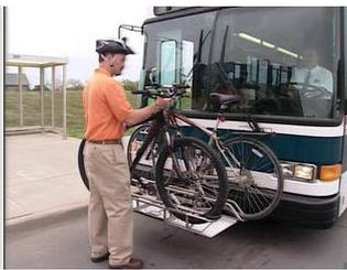
6. If there is a bike loaded in the inside slot on the rack, load your bike with the rear wheel facing the curb. **NOTE:** If the outside slot is occupied; slide the bike from the curb side, rather than trying to lift your bike over the other bike into the inside slot.
