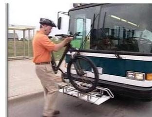
**4. If the rack is empty, always load your bike in the slot closest to the bus with the front wheel facing the curb. This is called the inside slot.**
