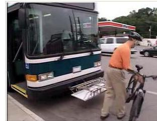
10. Lift your bike out of the rack. If the rack has two bikes and yours is loaded in the inside slot, release and lower the support arm and slide the bike toward the curb to remove it; instead of lifting it over the bike in the outside slot.
