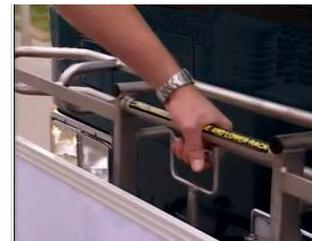
**3. To lower the rack, pull up on the handle and pull down. You only need to use one hand. Do not lean the bike against the bus.**
