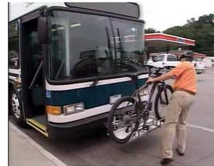
9. Lift the support arm and fold down.
